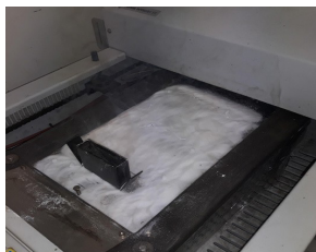
A thick layer of 5744 placed on top of solder surface.
